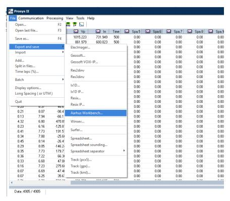
The output as a column based text file which included all data and waveform information needed for import into Aarhus Workbench.
